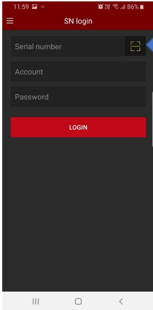
Click this symbol to open the camera on your smart phone, then scan the QR code that is displaying on the IP camera configuration screen.
